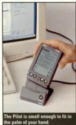
than a pack of cards, and weighing about 5.7 oz. with its two AAA batteries (which, incidentally, last about two months with regular use), it fits just about anywhere.
