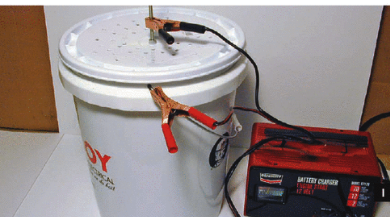
Fig. G: Put the mesh ring into the bucket and thread the conductor wires through the hole in the lip of the bucket. Fig. H: Put the rusty object on the hook and submerge in sodium carbonate solution. Fig. I: Connect the red
