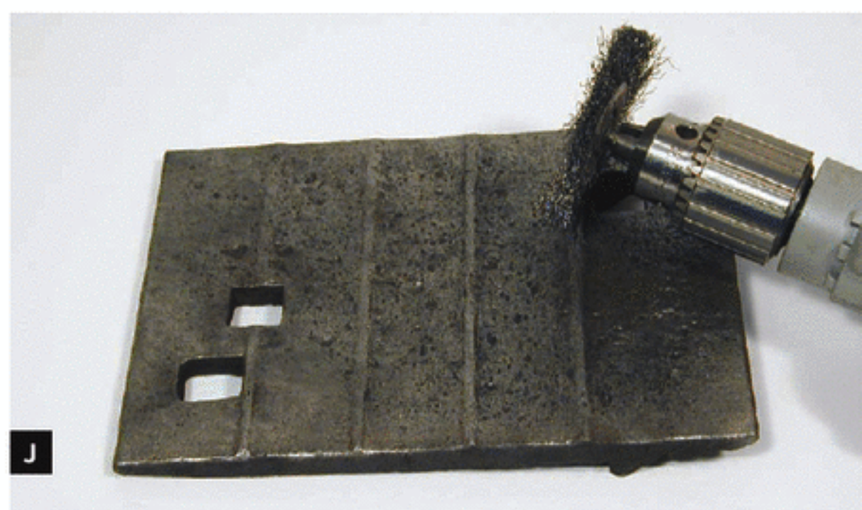
cable to the anode wires and the black cable to the rod in the lid. Fig. J: The scale and surface rust will be converted to a black powder that can be removed with a wire brush, wire wheel, or light abrasive blasting.
