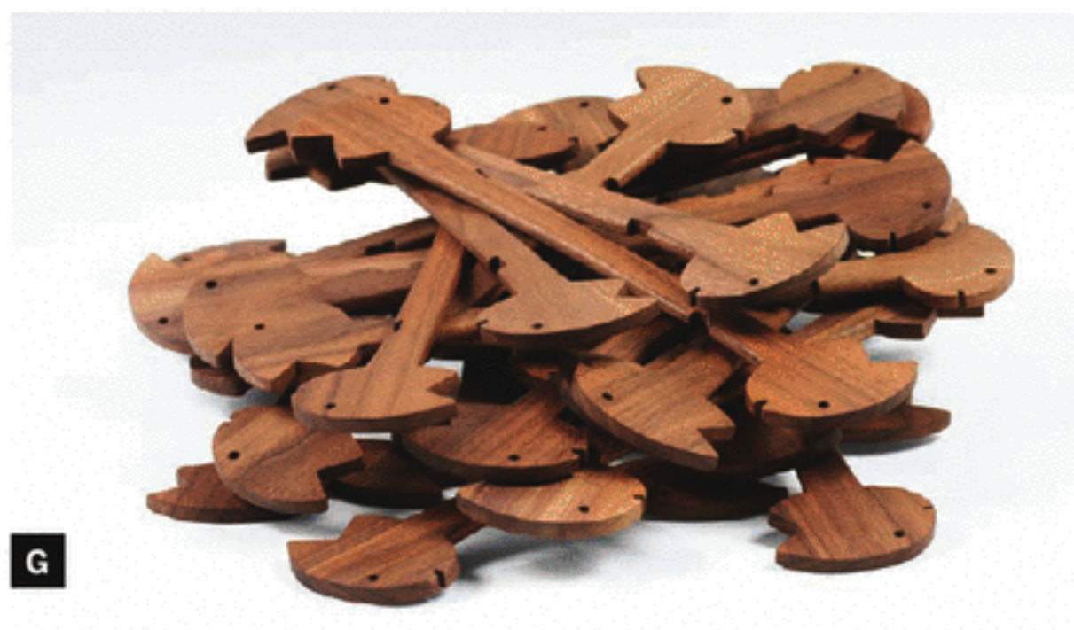
Fig. E: Drill 2 eye holes in each part. Fig. F: Cut one of the parts in half, as shown. This is the puzzle's "key" part, which will be added last. Fig. G: Apply an appropriate wood finish, e.g., tung oil, and allow it to harden.
