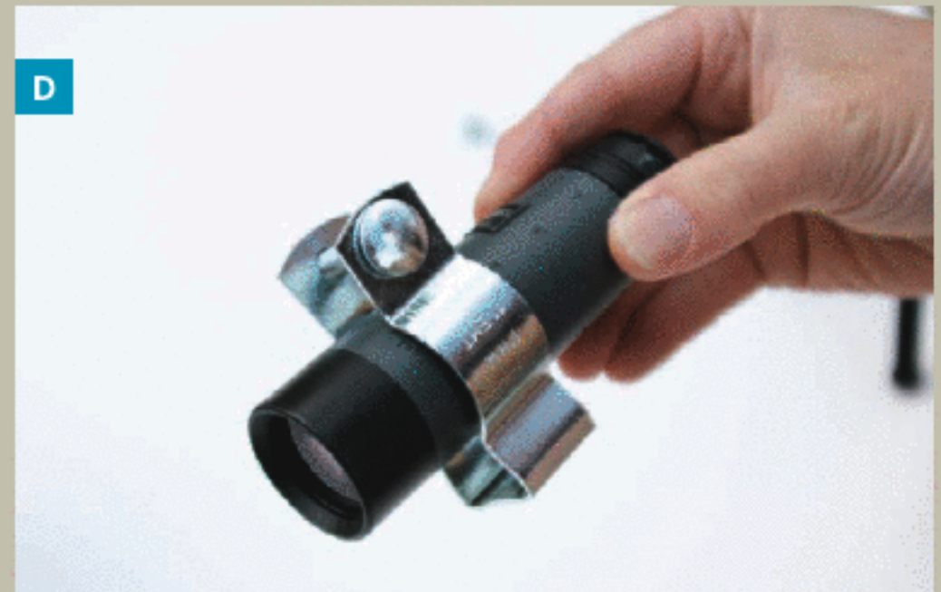
Fig. C: Attach the mini-tripod to the cellphone holster with the mount screw. Fig. D: Mount the monoscope using a 1" pipe clamp.
