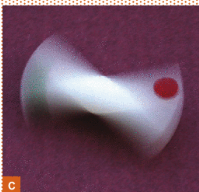
WHERE DID THE GREEN DOT GO? Fig. A: The spinning cylinder revolves around its midpoint (radius R ) and simultaneously around its long axis (radius r ). Fig. B: A small plastic cylinder has a red dot on one end, and a green dot on the other. Fig. C: Immediately after spinning, the motion is chaotic. Fig. D: As the cylinder stabilizes, many red dots are visible. Fig. E: When the spinning has stabilized, 4 red dots are clearly visible. The green dot is not visible.
