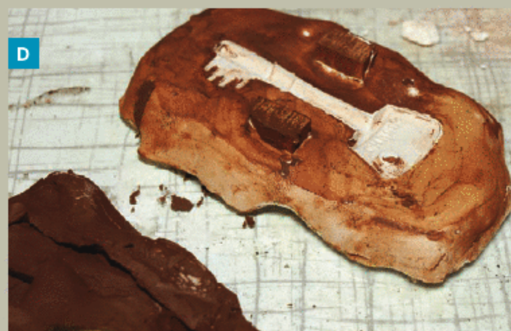
Figs. B–D: Make a mold using casting plaster (as shown here) or resin. Be sure to spray light oil or mold release into the mold before using it.
