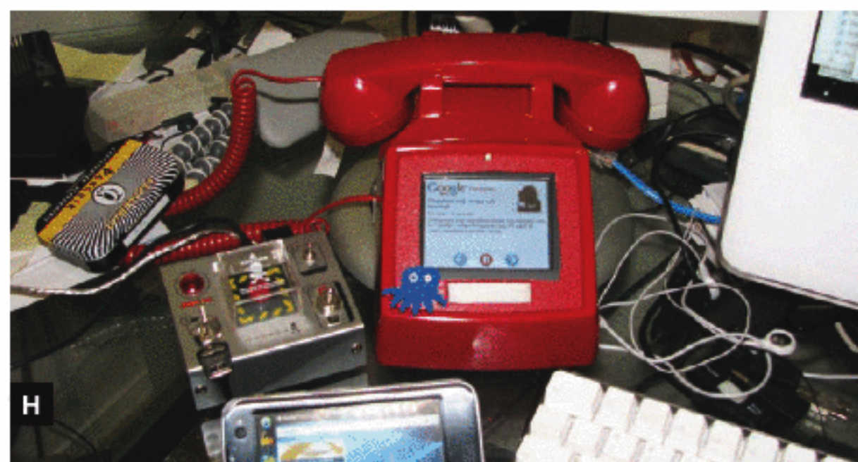
speakers fit nicely at each end of the handset. Fig. H: All done. It's fun to have a big, retro, important-looking red phone that runs Linux, tunes internet radio, and displays web information widgets.
