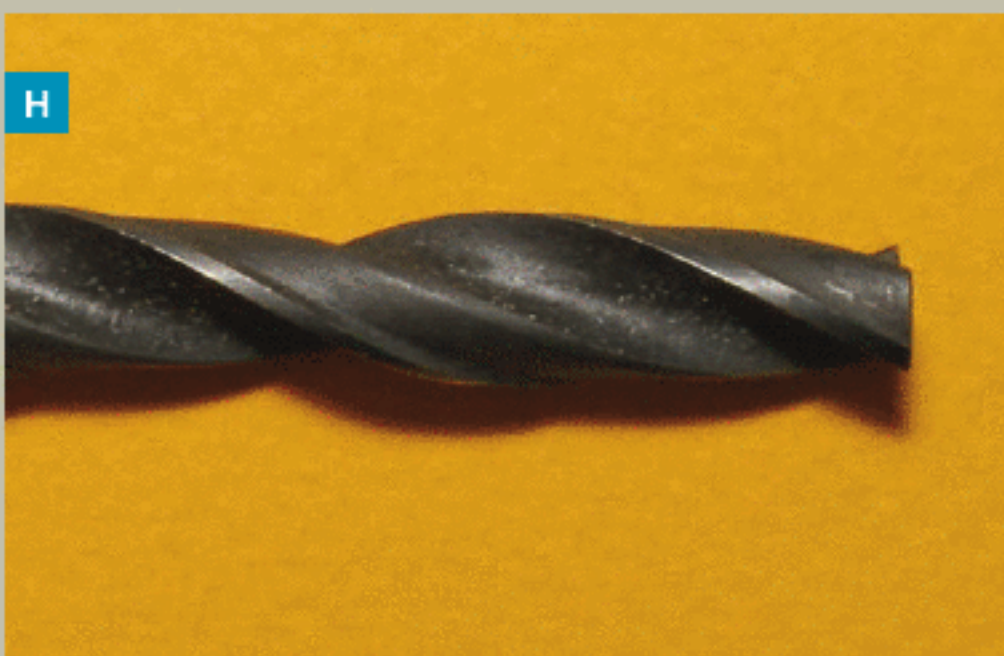
Fig. G: Drilling and tapping the bolt head is tricky, because the head is shallow. Use the depth stop on the drill press. Fig. H: Make a bottom drill from a twist drill.
