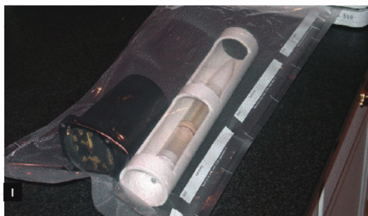
Fig. H: Calibrate the G-meter by stacking washers in multiples of carry load. Fig. I: Calibrate the altimeter alongside a working barometer or altimeter in a vacuum.
