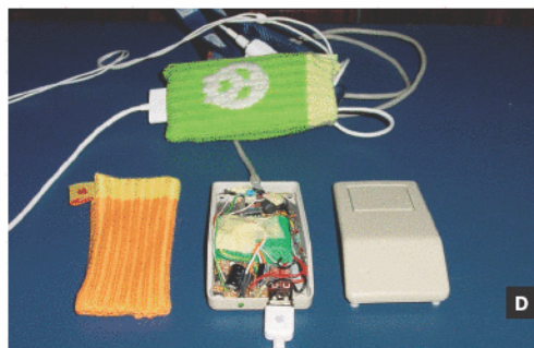
Fig. A: Bike-powered iPod charger detaches easily for parking. Fig. B: Original 6V hand-cranked charger with voltage stepped down to 5V for USB. Fig. C: Mouse case contains charger electronics and connects to bike dynamo via S-video plug on handlebars. Fig. D: iPod, opened-up charger, and iPod socks. Fig. E: Charger electronics, battery, voltage regulator, and USB port packed inside mouse case.
