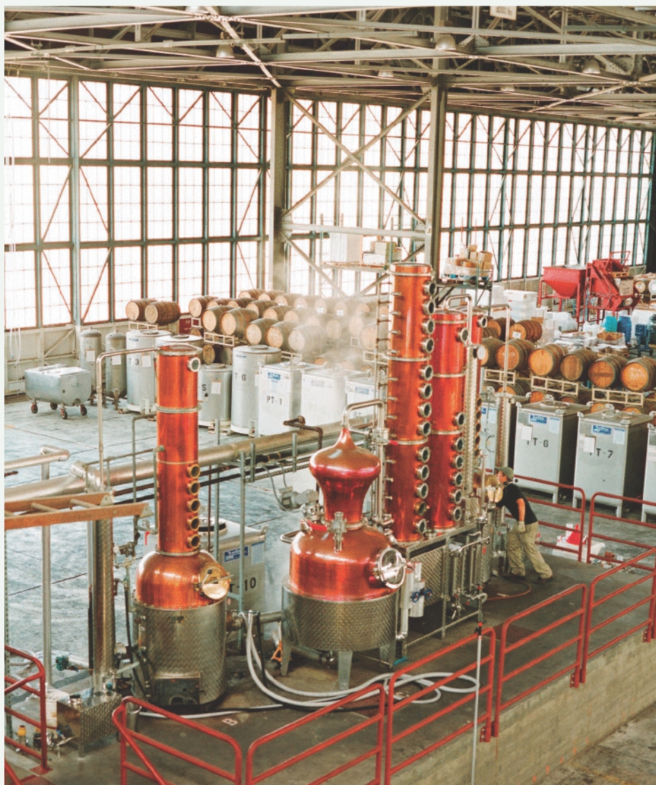
ABOVE: Three German-made pot stills on the main hangar floor produce vodka and eau de vie. BELOW: Bottles in Winters' office hold rare ingredients to add to his potions.
