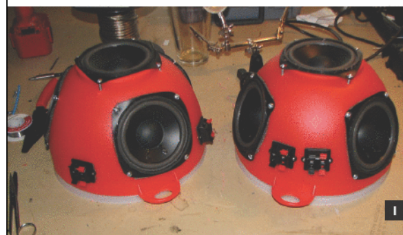
Fig. G: Speaker bolted in with washers and locking nuts. Fig. H: Terminal connected to the side of the bowl.
