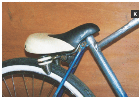
Fig. I: Plates welded to the gooseneck. This design lets you keep the handlebars original, rather than clamping them to a single top plate somehow. Fig. J: Seat clamp welded above the rear wheel.
