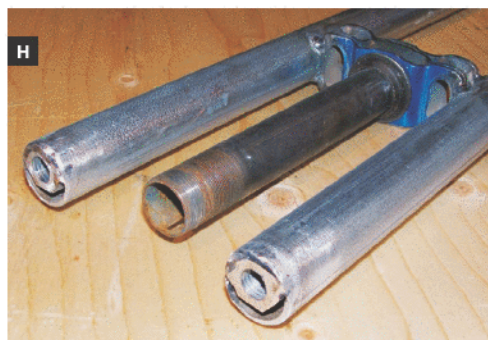
Fig. G: Cutting the gusset pattern. A jigsaw is better for tight curves, but this method works faster and makes good use of a worn cut-off wheel. Fig. H: Nuts welded into the fork legs.
