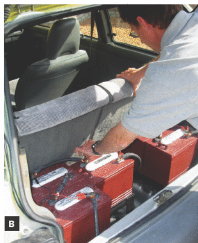
Fig. B: To run the motor, Weber uses eight 6-volt batteries, for a total of 48 volts. Three of the batteries (not shown here) are in the front engine space.
