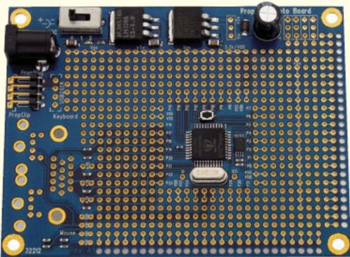
ABOVE: Gaming guru Andre LaMothe's Hydra Game Console (hydraconsole.com) is the first commercial application based on the Propeller chip. BELOW: The Propeller Proto Board can be used for permanent projects.
