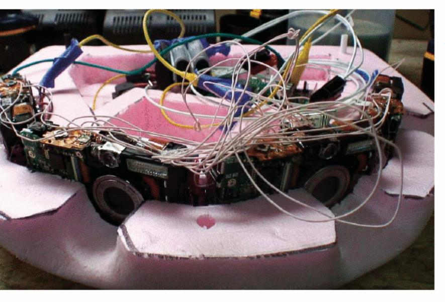
FIVE SNAPS UP: Four cameras point outward to capture a 180° panoramic image from space. Using the MAKE Controller, they take a picture every 7 seconds. A fifth, hacked CVS camera on the bottom gets the first 20 minutes of flight on video.
