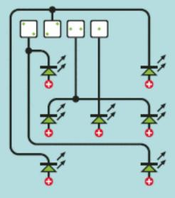
Seven LEDs are arranged in this pattern to emulate the spots on a die. The dice icons indicate inputs that correspond with outputs from the circuit in Figure 4.
