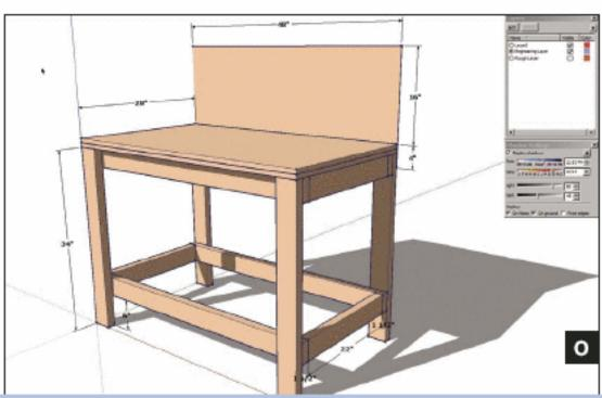
Fig. M: Cut two plywood sheets for the top.
