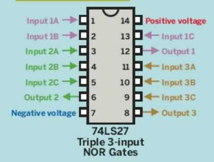
This chip contains three NOR gates with three inputs each. All inputs for each NOR gate are functionally identical.
