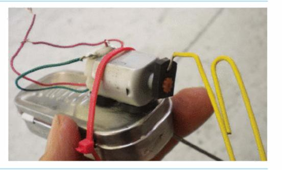
To operate the Vibrobot, twist the loose battery wire and the loose motor wire together (you can also solder an alligator clip to one of the wires for a switch). Experiment with the critter by gently bending the paper clip and legs into different shapes and observing the effects. Watch a video at makezine.com/10/123\_vibrobot.
