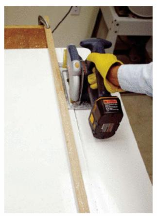
For smaller cuts, a band saw is trouble-free. Since ABS is soft, you can also use hand tools with very little effort, especially a Japanese-style, pull-to-cut saw, which makes exceptionally clean cuts. When pulling it, be careful that it doesn't jump out of the cut and across your hand.
