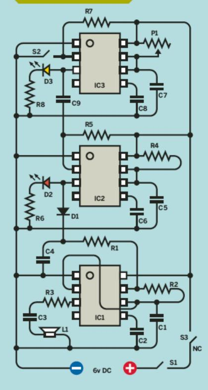
R1 through R6: Unchanged R7:  $10k\Omega$  R8:  $600\Omega$
