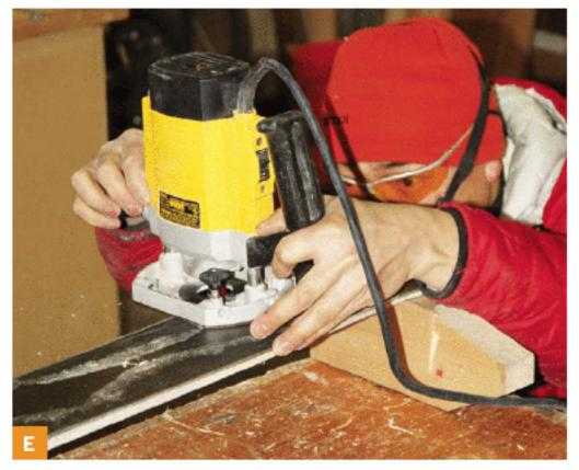
Fig. D: When they come off the press, the skis are attached to each other by the fiberglass sheet. Fig. E: Using a router to shape the sidewalls.
