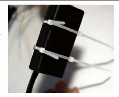
NOTE: Using 2 short cable ties instead of 1 long one makes it cleaner to go around corners.
