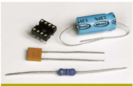
Fig. 3: Socket, big and small capacitors, resistor (front).
