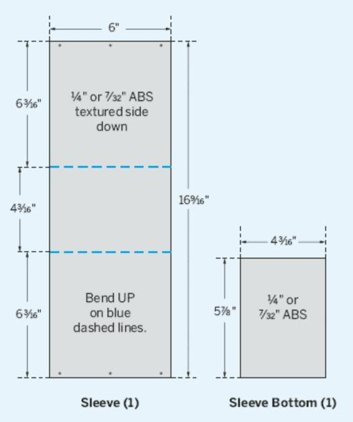
Drill holes 3/32" diameter, centers 3/16" from each edge, offset horizontally 1/2" from each corner.
