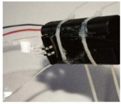
5c. Route the 4 wires from the LEDs and 2 from the battery pack along the top of the glasses toward the left temple (where they will connect to the PCB), twisting them together along the way. Keep the 2 wires from the battery pack together, so you don't confuse them with the LED wires.
