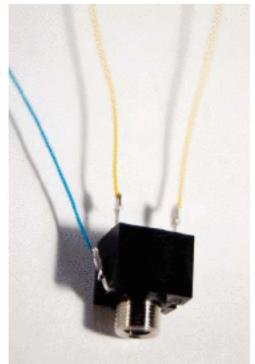
2e. Twist these 3 wires neatly, but leave about 1/2" untwisted. Cut them so that they all extend the same length, strip 1/32" off each, and tin. Solder the ground wire (blue) to the PCB trace that connects all of the LED grounds together. Then solder the right and left speakers (yellow) to the outputs for LED3 and LED4.
