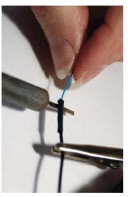
NOTE: Although you can use electrical tape to cover the exposed wires, heat-shrink looks nicer and won't unravel.
