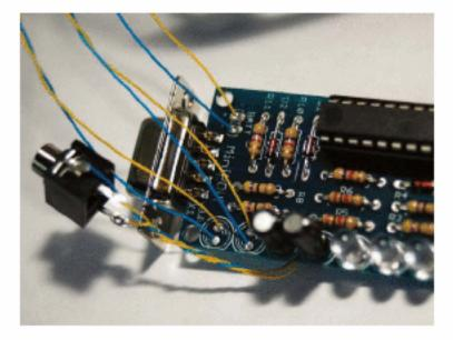
NOTE: Test the LEDs by turning on the battery pack power switch. The LEDs on the glasses should flash. If not, then double-check the wiring.
