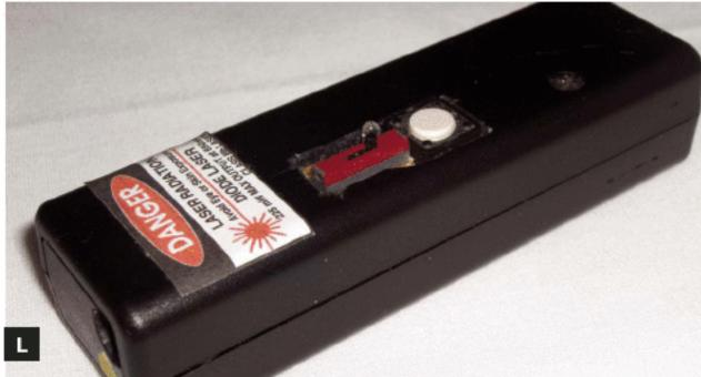
Fig. I: Laser diode wired in Digi-Key housing.
