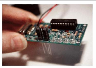
NOTE: Adding the capacitors and resistors creates low-pass filters that smooth out the square waves into sine waves, for more pleasing audio.
