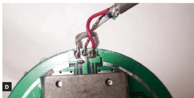
Fig. C: Waveguide with coiled wire mounts. Fig. D: Waveguide cable wiring to PCB.
