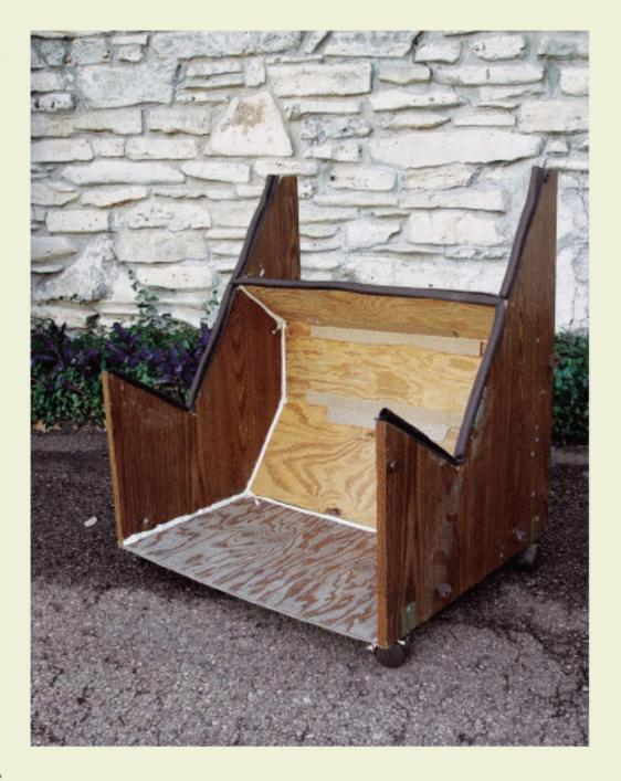
Sound comes out the back of the amp and is forced out the front of the stand. Beyond that, the shape of the barrier isn't too important. Be sure that the horizontal bit hits the amp's back above the speaker opening and below any controls.
