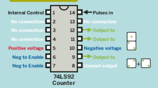
The 74LS92 counter requires power on Pins 5 (positive) and 10 (negative) and negative voltage on Pin 7 to enable it. Pins 9, 11, and 12 can be connected through transistors to LEDs representing spots on a
