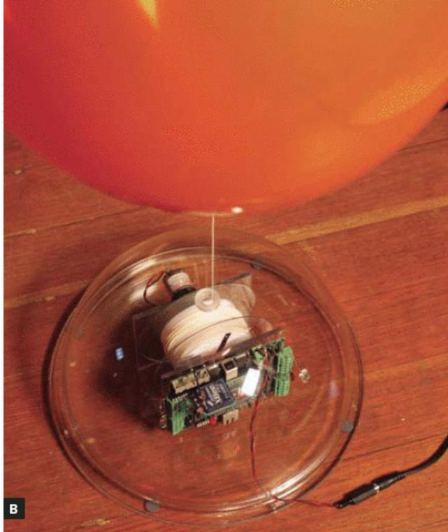
Fig. B: This balloon controller is based on the diVA project (makezine.com/go/diva), which hides the complexity of devices such as the MAKE Controller and makes it easy for people to control things through a web interface.
