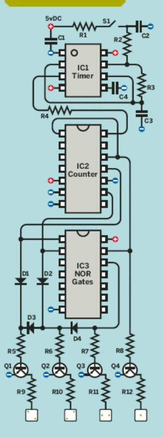
Each dice icon indicates an output that should be connected to the LED display.
