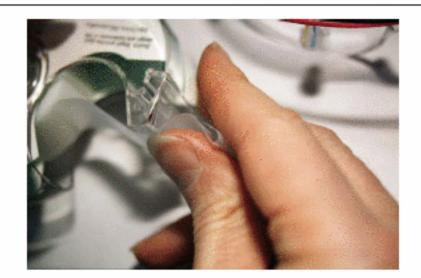
NOTE: Doubling the ends over makes it much easier to pull off the tape strips after the adhesive hardens.
