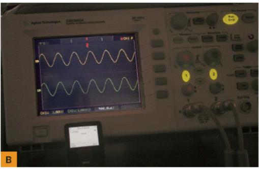
on the front panel. A knob for each channel adjusts the volts/div (volts per division) scale of the graph, and turning it to "1" sets the horizontal gridlines 1V apart, going up and down. The baseline voltage is controlled by another knob, labeled Position or Vertical Position. This lets you move the trace up and down. You can use these knobs to look at more than one trace at a time, adjusting the displayed voltage ranges for each channel to superimpose them against one another.
