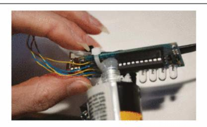
NOTE: Gluing the wires and terminals will prevent shorts and provide strain
