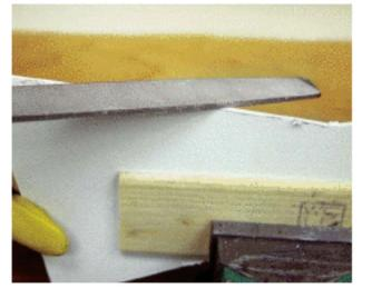
TIP: Saw slightly outside of each line, so that if the blade wanders you can use a coarse metal file to straighten the edge afterward.
