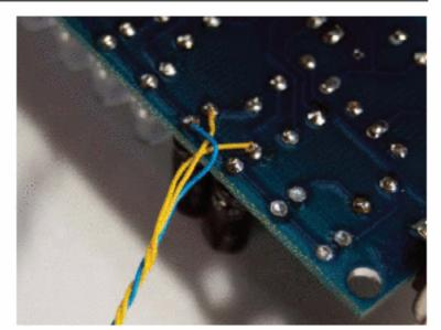
2f. Test the audio by plugging your headphones into the jack, putting them on, and flipping the power switch. You should hear some spacey sounds in both ears. If not, the most likely problems are bad solder connections or solder bridges.
