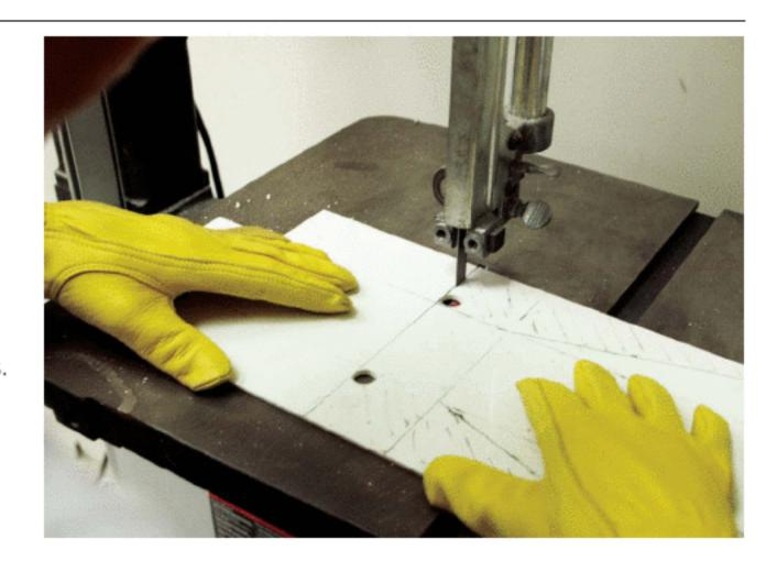
**3c.** Cut out the piece. After drilling the holes, cut around the edges of the shape using a band saw, hand saw, or jigsaw. The plan shows some of the outside corners rounded, in addition to the inside corners, but this is a matter of taste.
