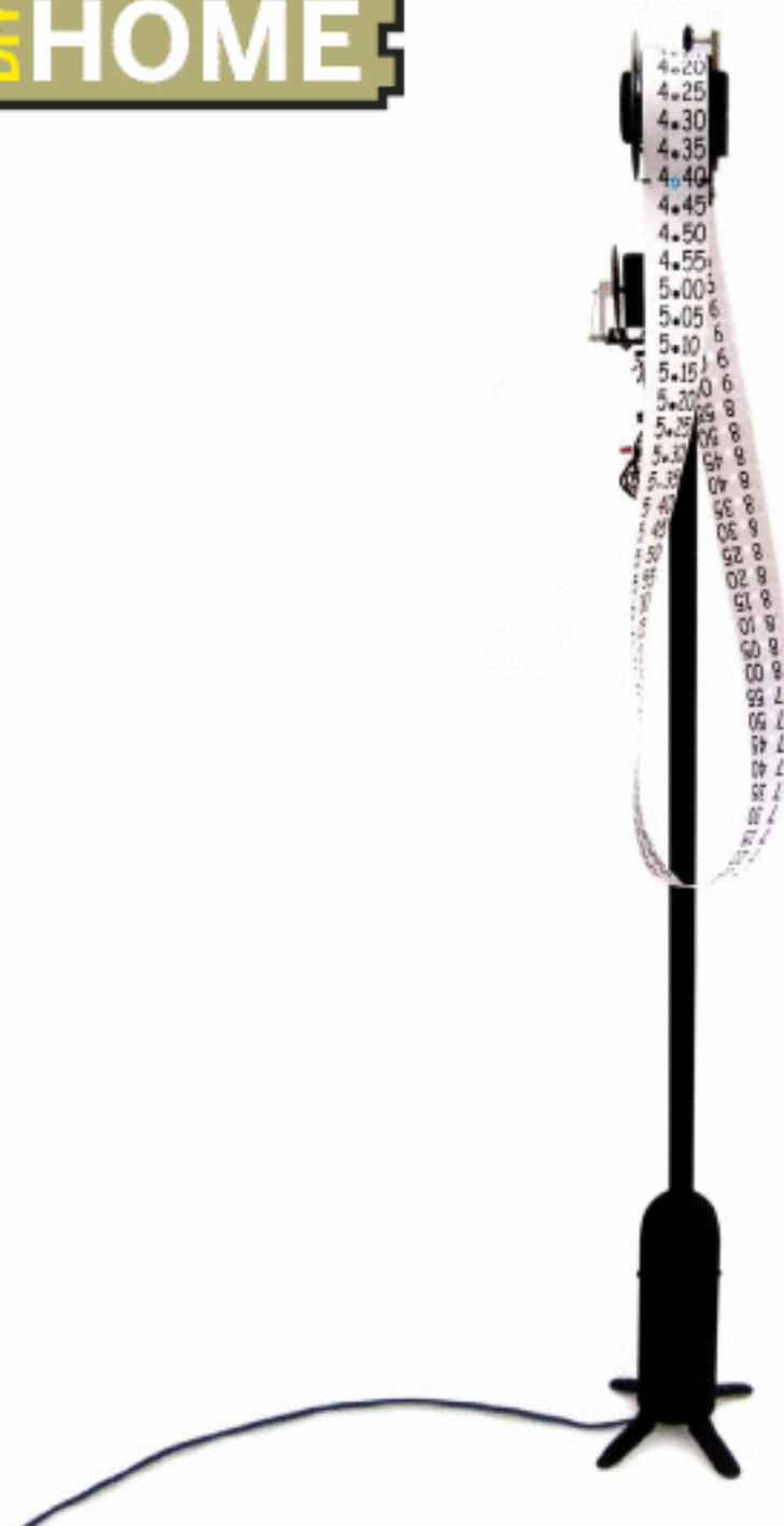
Fig. D: Moebius clock advances a single-sided paper loop with printed times. Fig. E: Dual-dial clock shows hours above and minutes below; hands swing back at the ends of their arcs.
