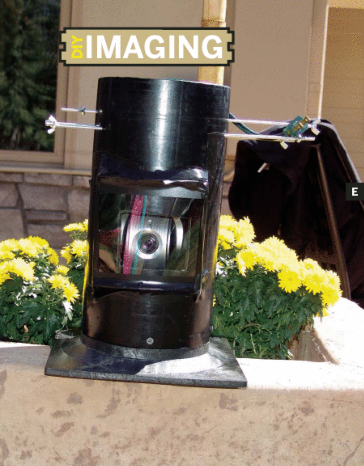
Fig. E: Portable webcam assembly can be hung under eaves or placed freestanding, weather permitting.
