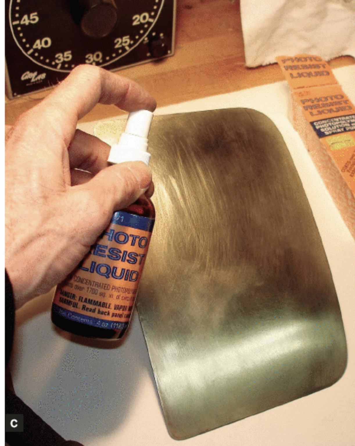
Fig. C: Sensitize the metal by coating it with photo emulsion liquid. Keep the spray bottle out of the light when not in use.
