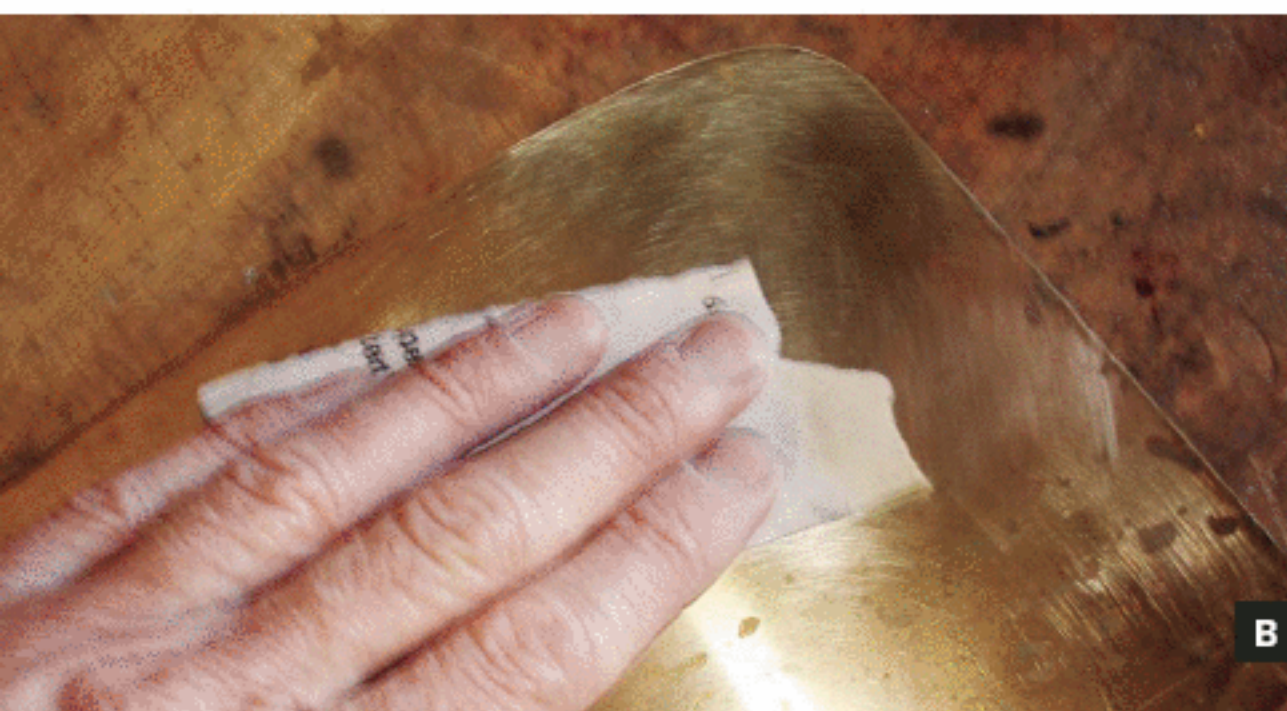
Fig. A: Print the etch image backwards onto a sheet of transparency film. Fig. B: Clean and polish the metal (copper or brass) surface. A single fingerprint can ruin the transfer.
