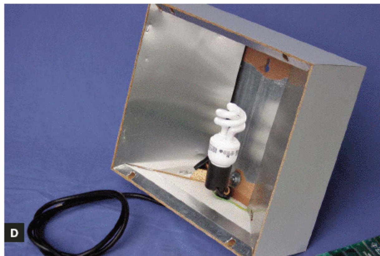
Fig. C: Removable light box back with lamp socket and compact fluorescent. Fig. D: The sheet aluminum lining stapled into the box reflects and diffuses light.
