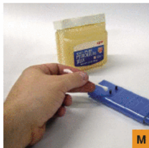
Fig. L: Set screw insertion. Fig. M: Lubricate inserts. Fig. N: Nut forming. Fig. O: Raw carbon trim. Fig. P: Clay insertion. Fig. Q: Epoxy spreading. Fig. R: Clamping.
