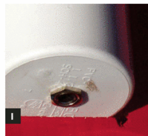
(3) Lag screws are used as strap buttons. Fig. F: Prepare the pickup by cutting away the top of the plastic case. Fig. G: Attach a rubber foot in the disk center. Fig. H: Drill the cap. Fig. I: Sand one side flat.
