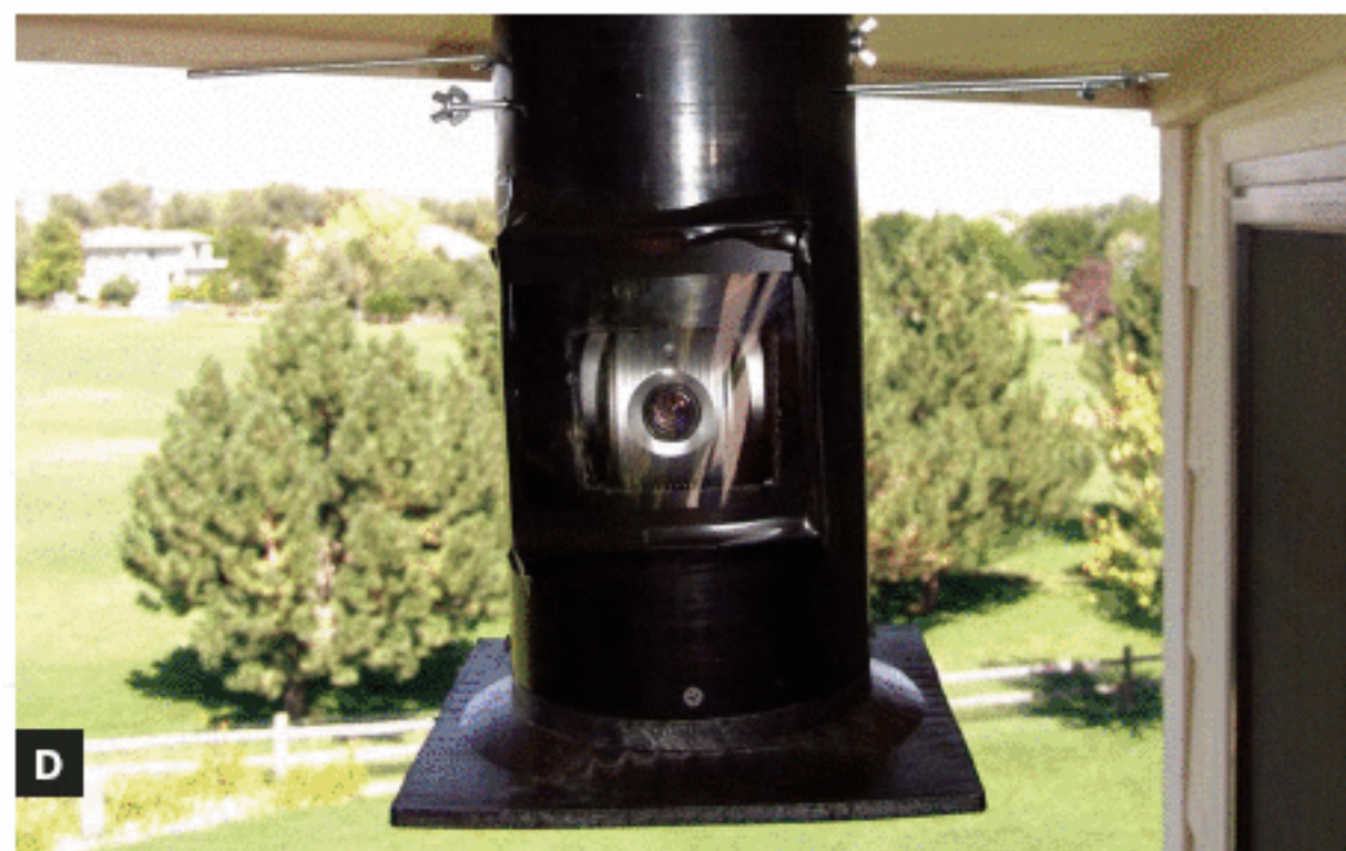
Fig. C: Internal view of webcam enclosure. Fig. D: Webcam assembly hangs from friendly neighbor's second floor balcony.
