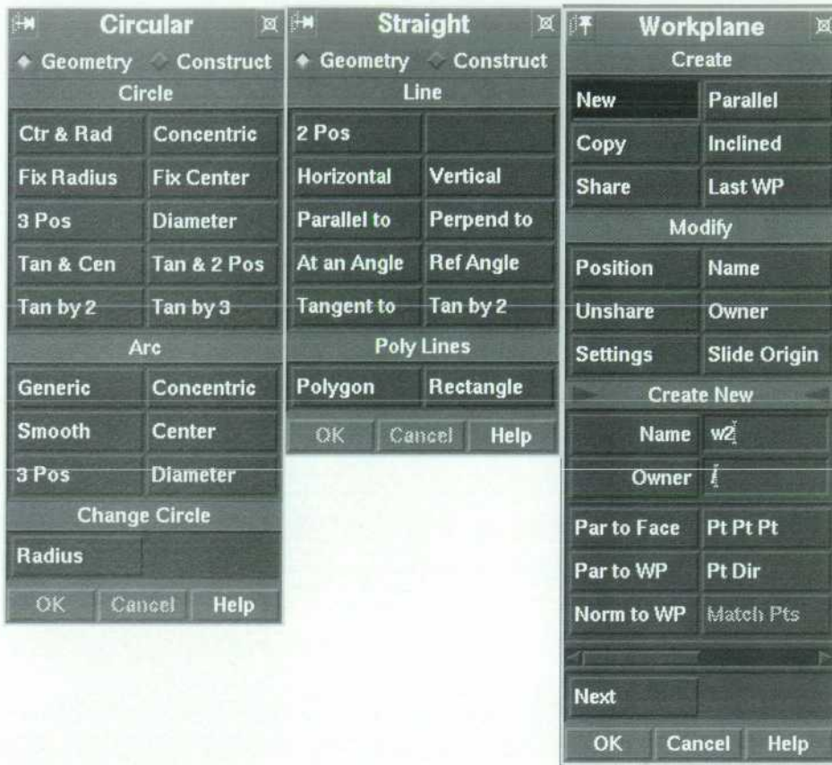
Fig. 2. Command dialog boxes with pin icons in the upper left corner. Two boxes are pinned to the screen and one is not.
