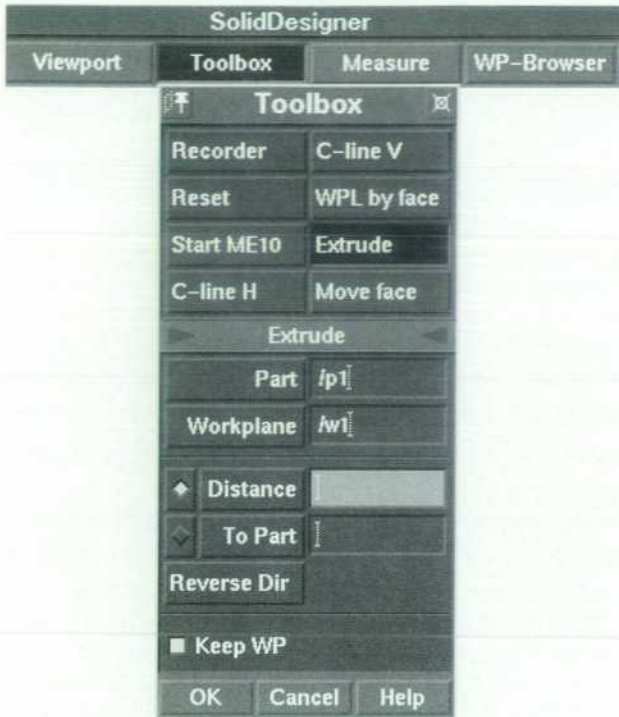
Fig. 7. The toolbox allows the user to build a custom command dialog box containing often-used commands.
