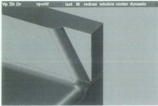
Fig. 16. The part of Fig. 13 changed by I-LOPs without the knowledge that there is a blended edge.
