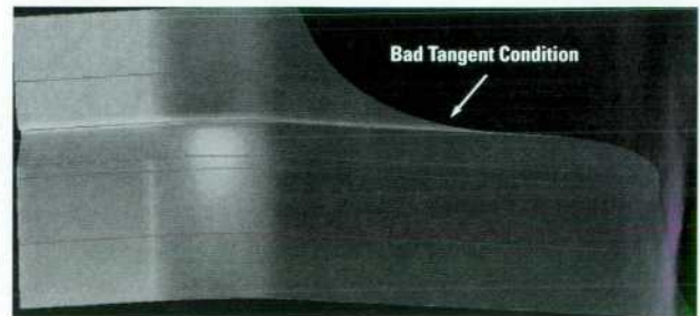
Fig. 17. Positioning too many profiles over too short a distance results in a wavy surface.
