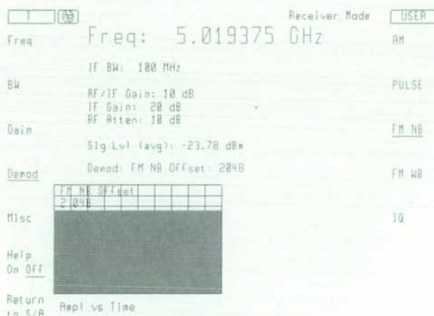
Fig. 5. The user interface screen provided by the HP 71910A receiver personality. The shaded area above is the time-domain display of an FM signal.
