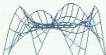
Fig. 27. WIREFRAME plot of the surface determined by z = x^4 - 4x^2y^2 + y^4 with view volume [-1,1] \times [-1,1] \times [-1,1] and eye point (4, -10, 3) .
