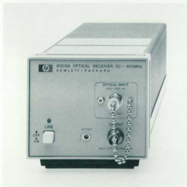
Fig. 1. The HP 81519A Optical Receiver converts optical power to electrical signals with a calibrated conversion factor of -1\text{V/mW} . It operates over an optical wavelength range of 550\text{ nm} to 950\text{ nm} and has an electrical bandwidth of dc to 400\text{ MHz} .
