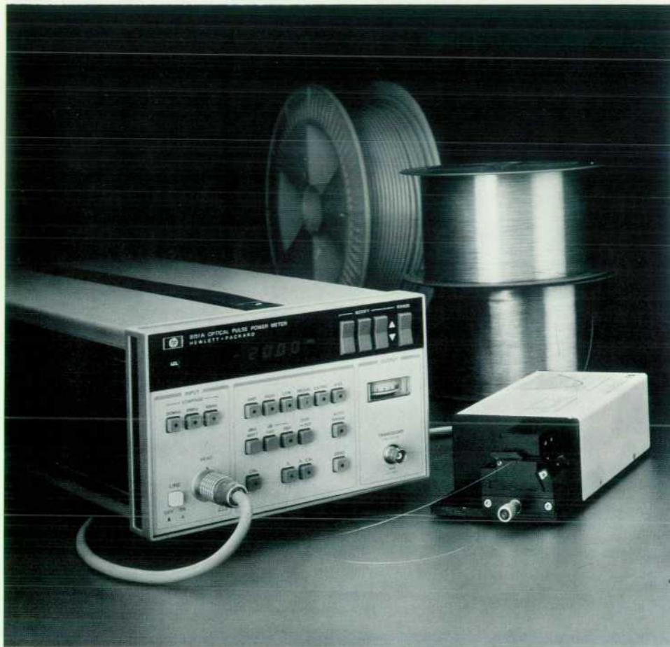
Fig. 1. The HP 8151A Optical Pulse Power Meter (left) measures and displays peak and average optical input power levels. It has a bandwidth of dc to 250 MHz for optical power between -20 dBm and +10 dBm. Its optical-to-electrical transducer is in a separate optical head (right) connected by a cable to the mainframe.
