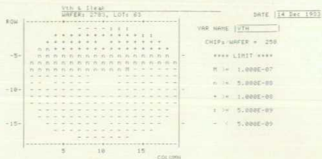
Fig. 5. Wafer map produced by the HP 4062A Parameter Test System.
