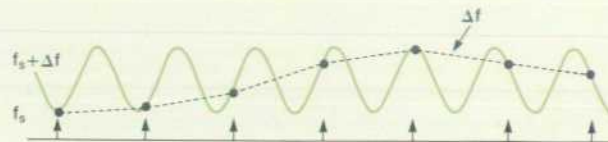
Fig. 2. When the input frequency is close to the sample rate f_s , the encoded result is aliased to the difference or beat frequency \Delta f .
