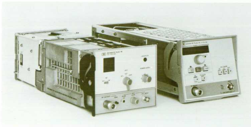
Fig. 3. Two types of plug-ins can be used in the 8350A Sweep Oscillator mainframe. The 83500 Series (right) is a group of high-performance plug-ins designed specifically for the 8350A. Existing 86200 Series plug-ins (left) can be used with the 11869A Plug-in Adapter (rear portion of unit at left).
