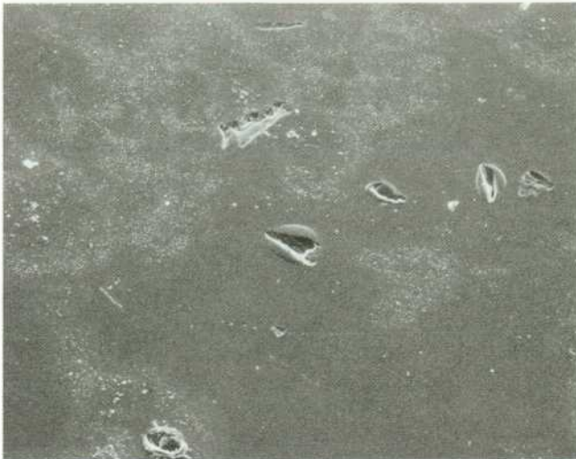
Fig. 3. Grit indentations in polyester film shown at a magnification of 80 \times .
