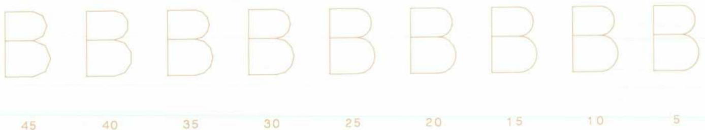
Fig. 6. Effect of chord angle on character quality. The letter B is drawn above for various selected chord angles. The smaller the chord angle the smoother the arcs and the longer it takes to write the character.
