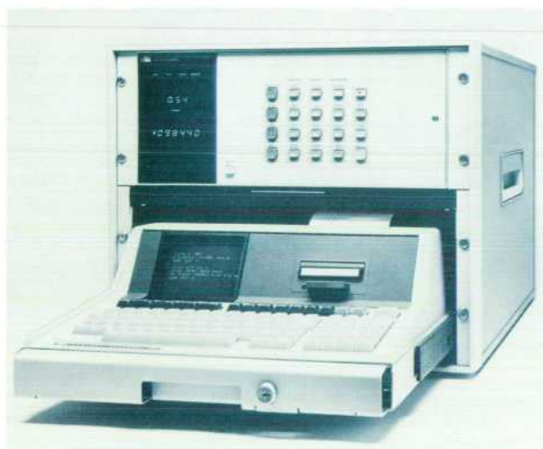
Fig. 1. The 3054DL system combines a 3497A Data Acquisition/Control Unit with various accessories and an HP-85 as the controller in a packaged arrangement for easy and convenient data logging. The system comes with extensive software for displaying and analyzing data, thermocouple voltage-to-temperature conversions, and configuring data logging setups.
