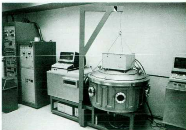
Fig. 2. ICPL's computer-controlled plasma systems were designed in-house to meet the requirements of VLSI processing.
