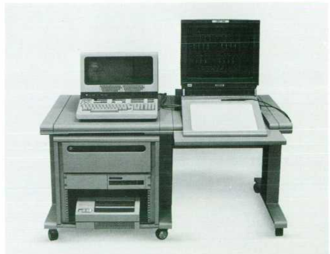
Fig. 1. IGS workstation consists of computer, CRT terminal, graphics tablet, and high-resolution color display.
