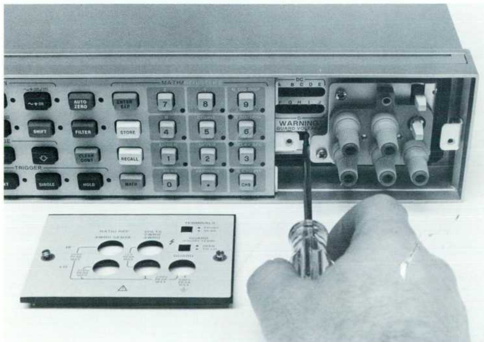
Fig. 14. All functions and ranges of the 3456A DVM can be completely calibrated from the front panel of the instrument by removing the cover at the right as shown.
