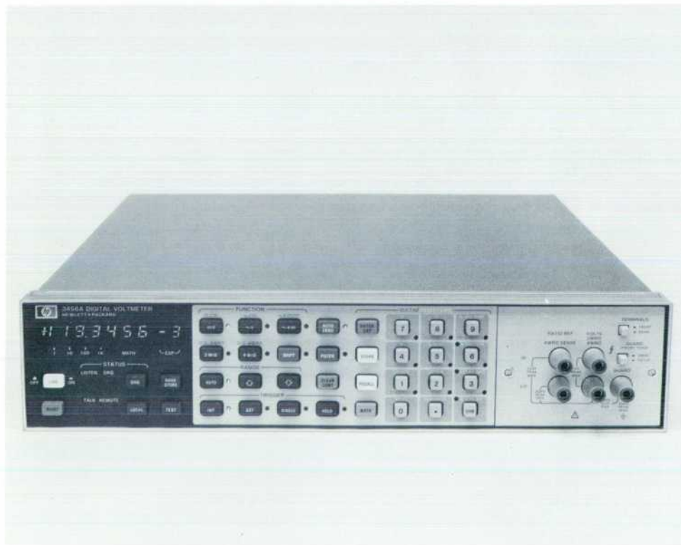
Fig. 1. The HP Model 3456A Digital Voltmeter is a 3½-to-6½-digit, fully-guarded integrating voltmeter with flexibility and precision, designed for both bench and system measurement applications.
