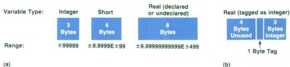
Fig. 1. (a) Each variable is allocated space in the memory according to its type specification. (b) If a REAL variable is perceived to be actually an integer of up to three bytes, it is stored in memory as shown and processed internally as an integer.
