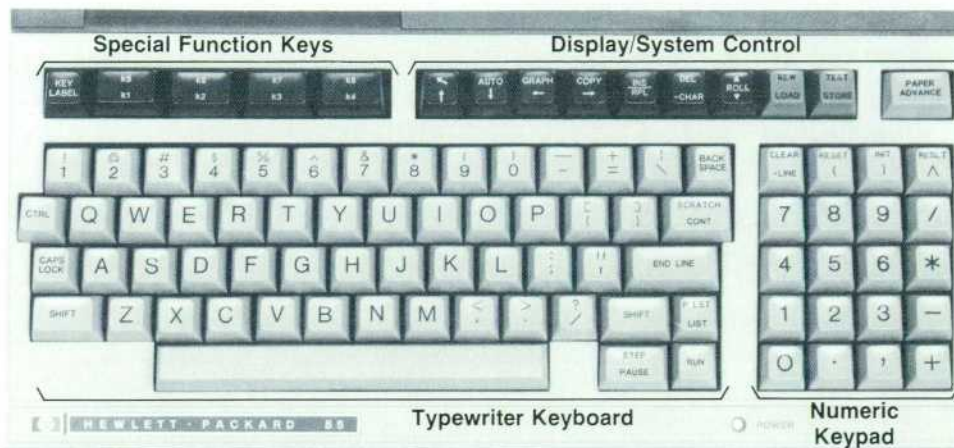
Fig. 4. The HP-85 keyboard is organized into four sections. Besides the normal typewriter section there is a numeric keypad for easy entry of data, a group of special function keys located close to the CRT display where their respective assigned labels may be displayed, and a set of control keys for frequently used system commands and editing/display control.
