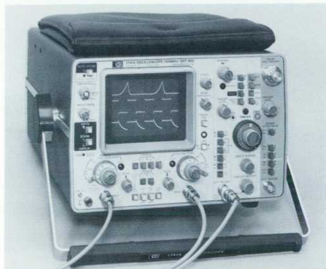
Fig. 1. Model 1741A is a portable, laboratory-grade, dual-trace 100-MHz oscilloscope that has variable-persistence and storage modes of operation with a writing rate of >100 \text{ cm}/\mu\text{s} . The most sensitive deflection factor is 5 \text{ mV}/\text{div} , expandable to 1 \text{ mV}/\text{div} on both channels simultaneously (with a reduction in bandwidth to 30 MHz). An external waveform used for triggering the sweep may be displayed on a third trace to assist the operator in selecting the trigger point.
