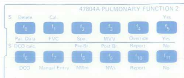
Fig. 2. An overlay labels the softkeys on the desktop computer, enabling any of the various pulmonary measurements to be initiated by pressing a single pushbutton.
