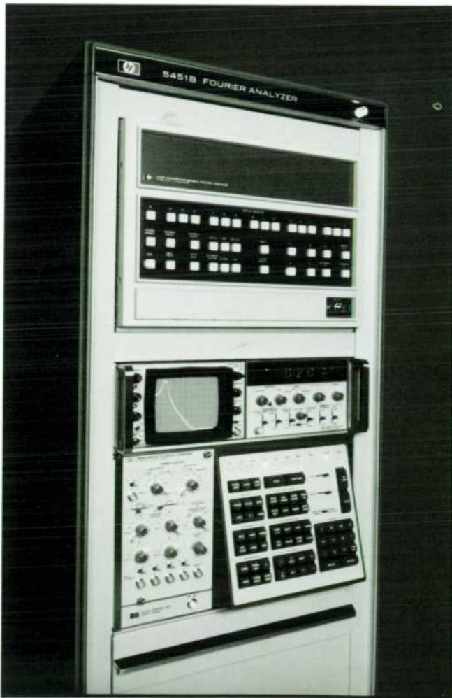
Fig. 9. Thanks to the microcode capability of the HP2100S computer, the 5451B Fourier Analyzer is ten times faster than the 5451A.
