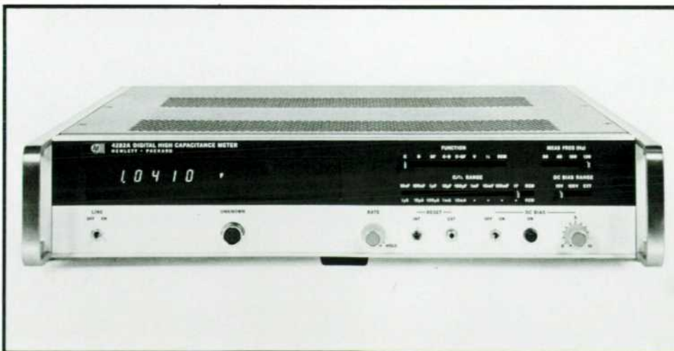
Fig. 1. Model 4282A Digital High-Capacitance Meter measures capacitance to one farad, dissipation factor to 10.00, the product of capacitance and equivalent series resistance ( \Omega\text{F} ), and dc voltages to 600V. An option adds leakage current measurements.
