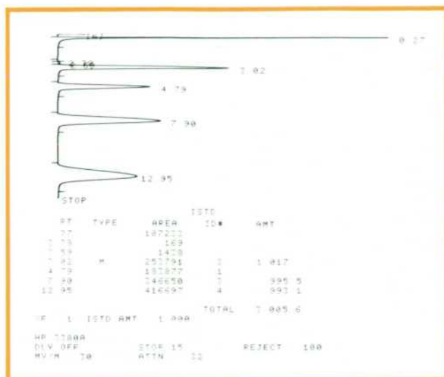
Fig. 4. Typical chromatogram and report generated by the Model 3380A Integrator. The retention time for each peak is printed alongside the peak. The analysis report is printed after the chromatograph run is completed. The final two lines give the settings of the integration controls.
