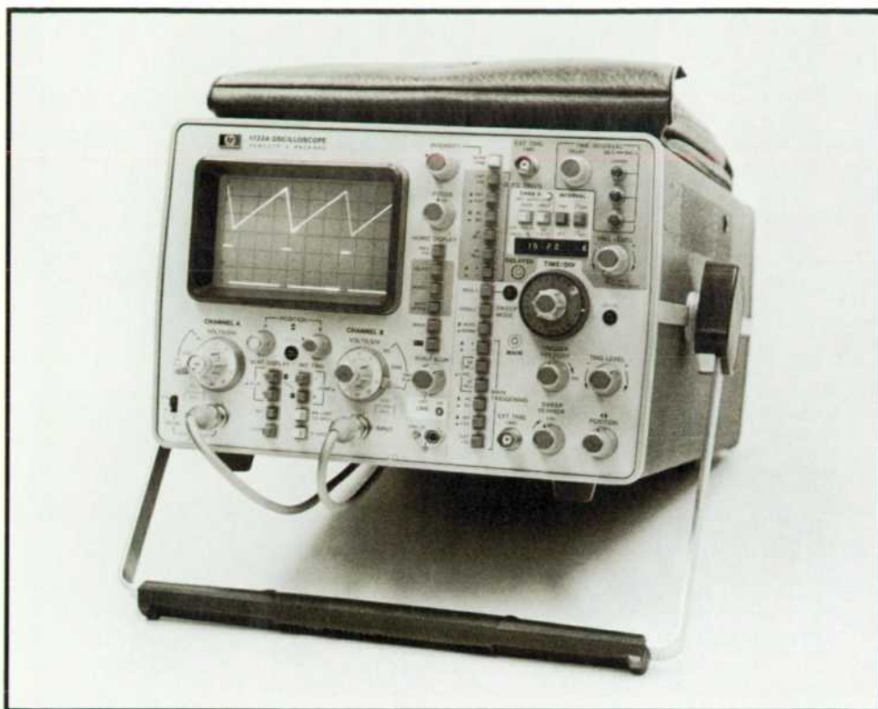
Fig. 1. Model 1722A Oscilloscope is a high-performance dual-channel instrument with 1.3 ns rise time, 50 \Omega or 1 M \Omega /11 pF input impedance, sweep times to 1 ns/div, and the dual-delayed sweep that provides higher accuracy, resolution, and convenience in time-interval measurements. Its LED display gives direct readout of time intervals, frequency (1/TIME), and voltage.
