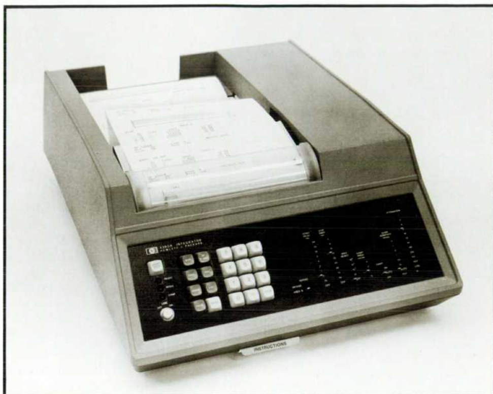
Fig. 3. Model 3380A Integrator records chromatogram and analysis on the same sheet of paper. Recording and integration are controlled by the slide switches. The keyboard is used only for computations related to calibration procedures.
