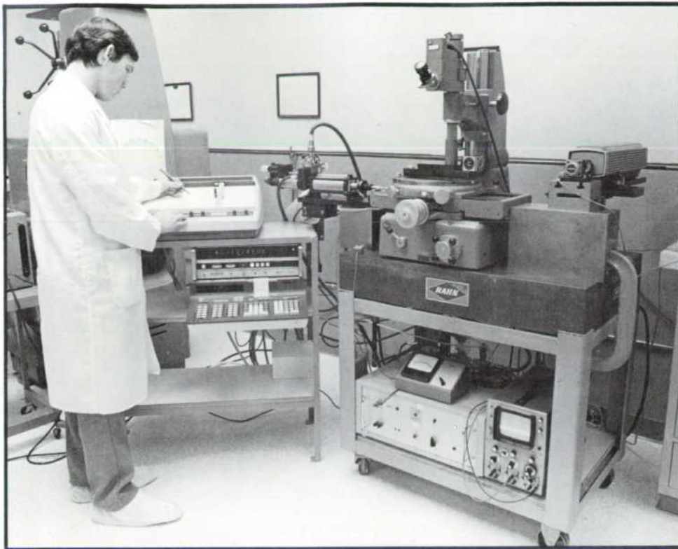
Fig. 2. Measuring system consists of toolmaker's microscope, photoelectric microscope tube, air motor drive, laser interferometer, calculator and plotter. The oscilloscope is used to monitor the photoelectric microscope output.
