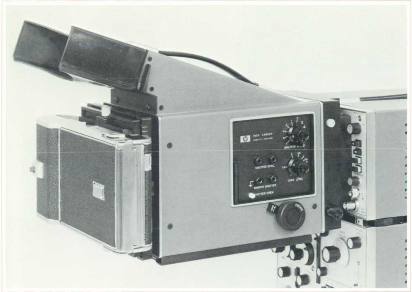
Fig. 1. Hewlett-Packard Model 195A Oscilloscope Camera mounts directly to HP 5-inch round and rectangular CRT bezels. Adapters, optionally available, fit Camera to most oscilloscopes of other manufacturers.
