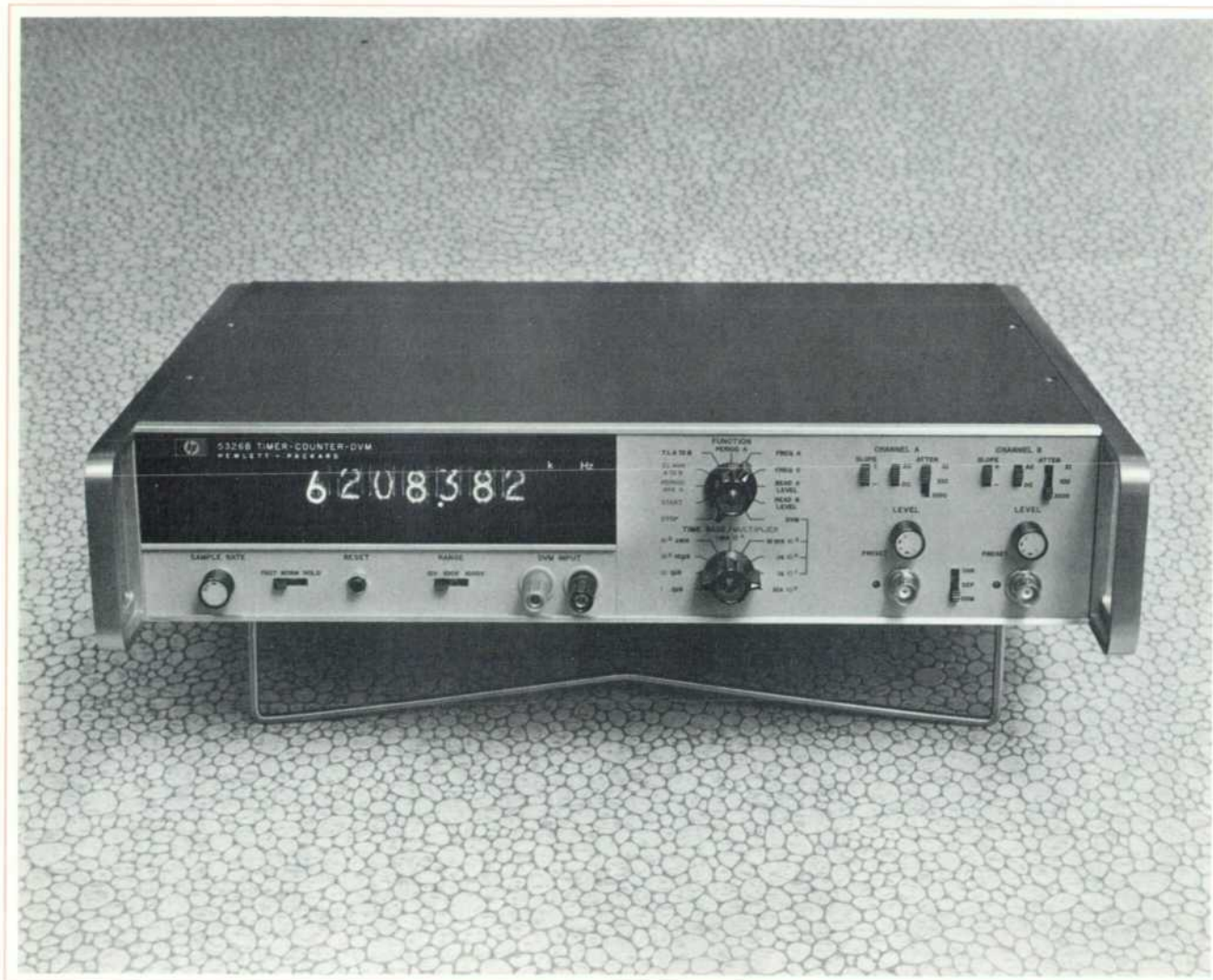
Fig. 1. Model 5326B Timer/Counter/DVM is a 50 MHz universal counter and a four-digit integrating digital voltmeter in one package. It has many new capabilities, most notably time-interval averaging and the ability to measure its own trigger level settings. Model 5326A is the same instrument without the DVM.
