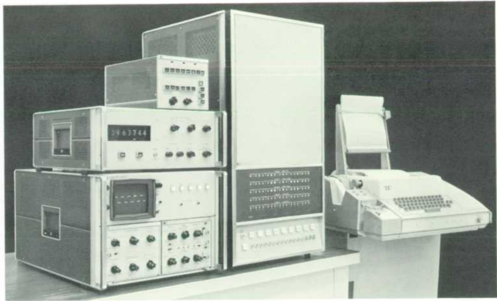
Fig. 3. Typical signal-analyzer/computer system contains HP 5480A Signal Analyzer for on-line signal processing, and computer and peripherals for off-line processing and storage. New Model 5495A I/O Coupler is instrument with digital display tubes. Small box on top of coupler is specially built program selector which provides pushbutton selection of computer programs listed in Table I.
