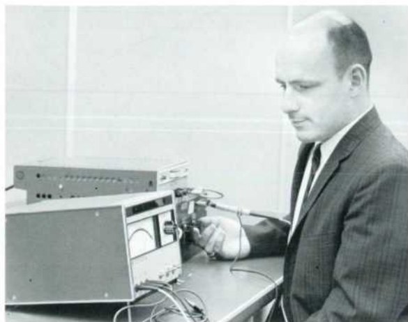
Fig. 6. New autoranging dc volt ohmmeter automatically changes measurement range whenever meter indication exceed 95% of full scale or drops below 25% of full scale. Autoranging speeds measurements in applications such as with dc resistance bridge shown here in which new instrument serves as null detector. Voltmeter switches ranges as required while bridge is brought to balance, thus avoiding overloading or pegging below zero.
