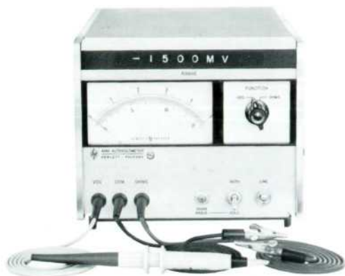
Fig. 2. New -hp- Model 414A Autovoltmeter switches to correct range in less than \frac{1}{3} -second after contact is made. Illuminated display shows range and selected function (volts or ohms). Mirror-backed, taut-band meter has individually-calibrated scales for high accuracy. Separate probes on 4-ft. cables are provided for voltmeter and ohmmeter functions.
