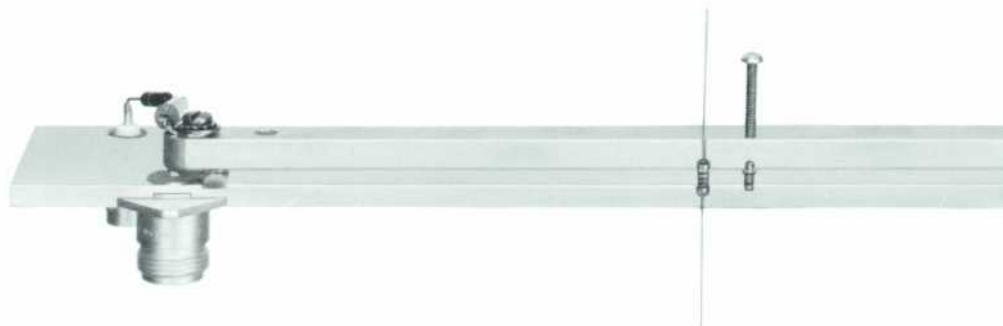
Fig. 8. Broadband stripline circuit used in bench work with Step Recovery Diode. Either glass or ceramic style diodes can be accommodated as shown.
