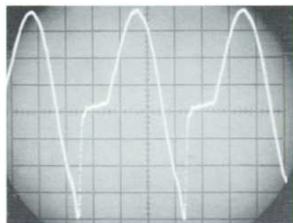
Fig. 5. Oscillogram of current through a Step Recovery Diode when driven by a sine wave (50 Mc). Abrupt transition on negative half-cycle occurs when stored charge becomes depleted and is an efficient mechanism for generating harmonics (Fig. 1).
