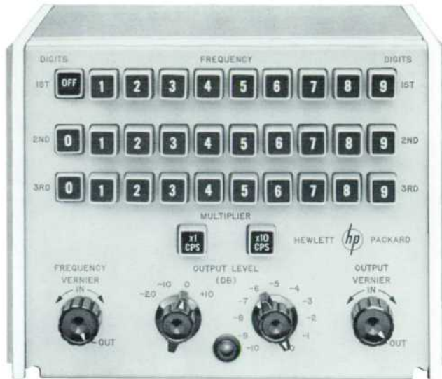
Fig. 1. Push-button oscillator for telephone test work operates from 10 cps to 10 kc with an absolute accuracy of \pm 0.2\% . Instrument matches 600- and 900-ohm lines, operates from -48 vdc supply.
