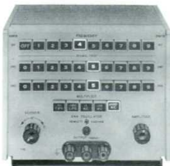
Fig. 4. Photograph indicating method of selecting output frequency in new oscillator. Buttons are set to give output frequency of 455 kc.
