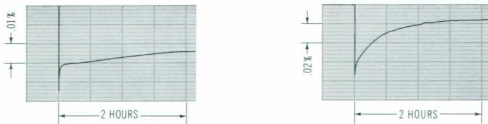
Fig. 6. Curves showing typical turn-on stability at room temperature of new Push-Button Oscillator. Left curve is at 100 cps, right curve at 100 kc.
