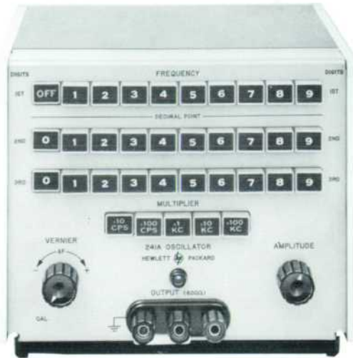
Fig. 3. Panel view of new -hp- Model 241A Push-Button Oscillator. Push-buttons permit selecting 4500 output frequencies from 10 cps to 1 megacycle (999 kc). Frequency vernier provides overlap between switch frequencies.
