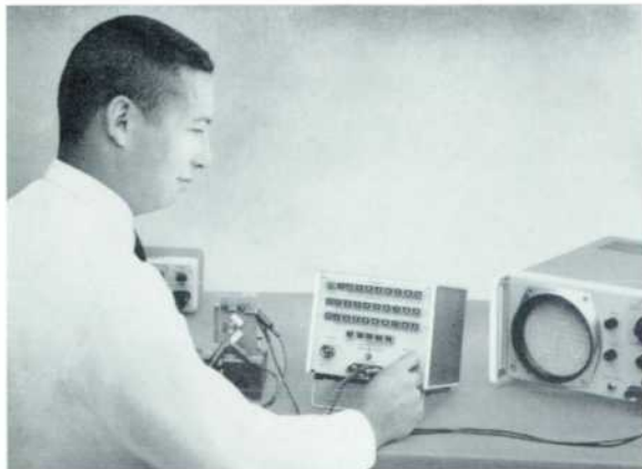
Fig. 1. New -hp- Model 241A Push-Button Oscillator operates from 10 cps to 1 megacycle, facilitates testing where repetition of often-used frequencies is desired. Push-button frequency selection has been used to achieve high repeatability of output frequency.
