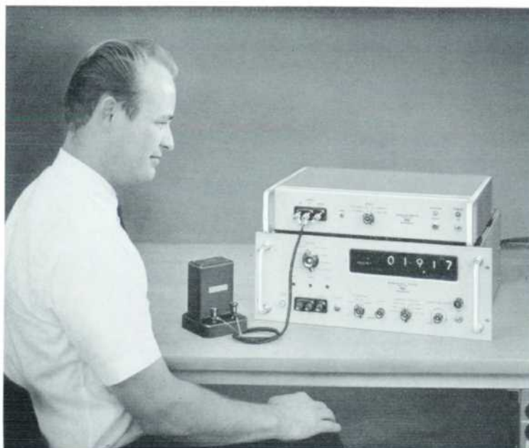
Fig. 1. Dymec Model DY-2411A Guarded Amplifier (upper unit) increases sensitivity of DY-2401A Integrating Digital Voltmeter by 10 times, permitting measurements to below 10 microvolts. Amplifier has input impedance above 10,000 megohms, here enabling stable measurement to be made on standard cell which is very sensitive to current drains even of microamperes. Reading is 1,019.17 millivolts with first digit off scale to left.
