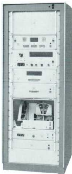
Fig. 5. DY-2401A Voltmeter and new DY-2411A Amplifier are incorporated in Dymec DY-2010G Thermocouple and Strain Gage Measuring System. System measures up to 200 inputs at 5-place full-scale sensitivity of \pm 10,000 millivolts. Measurements are recorded on paper tape by high-speed punch (open panel) for computer processing.
