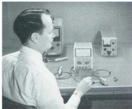
Fig. 1. New -hp- Model 410C Multi-Function Voltmeter has been designed as a general-purpose dc-measuring instrument which can also measure ac to 700 megacycles with detachable ac probe (shown at left of 410C in center). Instrument's high current sensitivity permits measuring small currents as in above photo, where diode leakage current of 1.6 nanoamperes is being measured.
