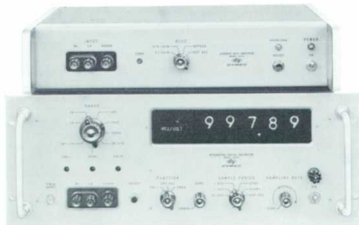
Fig. 4. Panel view of DY-2411A Guarded Amplifier with DY-2401A Integrating Digital Voltmeter. Inter-connections are at rear.
