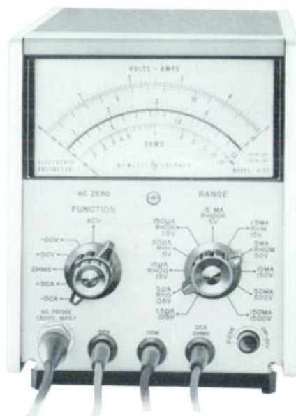
Fig. 3. New -hp- Model 410C Multi-Function Voltmeter measures dc voltage, dc current, resistance and ac voltage to 700 Mc (with detachable ac probe). Dc-measuring circuitry is floating to permit off-ground measurements.
