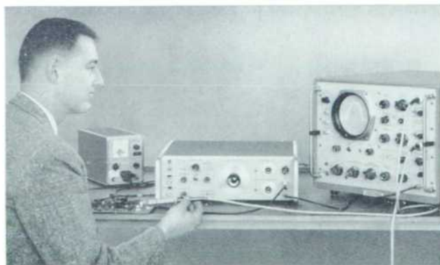
Fig. 1. New -hp- Model 215A Pulse Generator (in center) provides pulses as short as 1 nanosecond for general-purpose testing. Pulses are provided at high level and from direct-coupled 50-ohm source for simplicity of external use.
