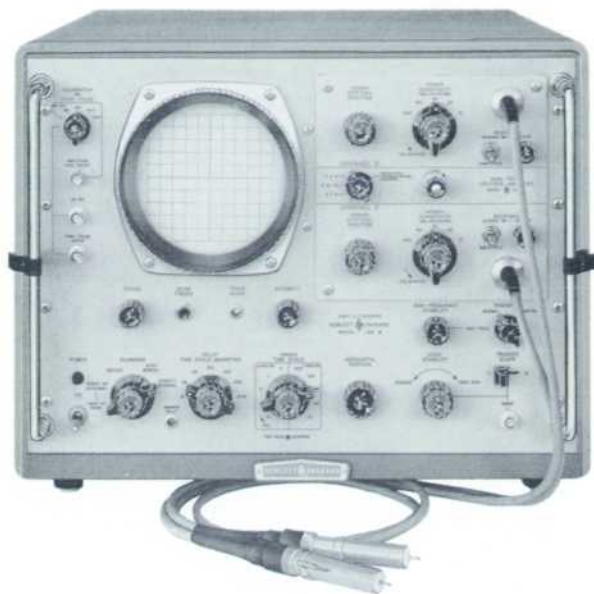
Fig. 10. -hp- Model 185B Sampling Oscilloscope with 0.35-nanosecond rated rise time used to make oscillograms appearing throughout this issue.
