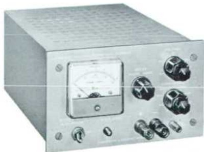
Fig. 1. Harrison Laboratories' Model 865B Power Supply is less than 8 inches wide, weighs only 12 pounds but supplies up to 0.5 amp at 0-40 volts. Any number of these compact supplies may be operated in series or parallel for higher voltages or currents. Either constant voltage or constant current mode of operation is possible.
