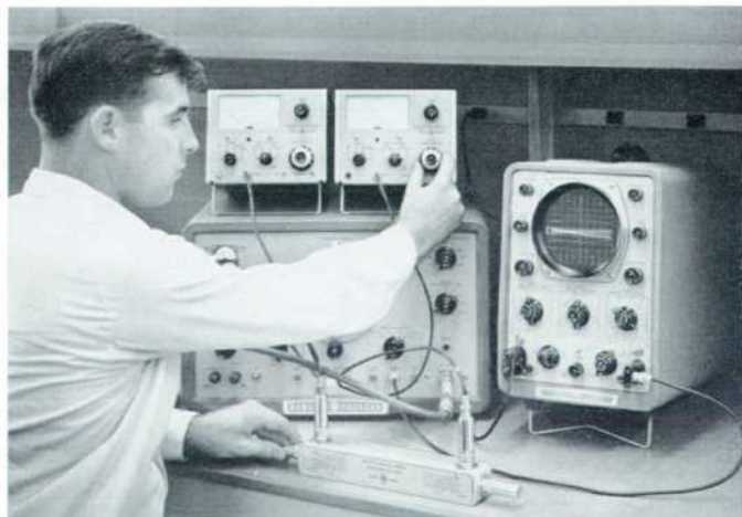
Fig. 1. New -hp- Model 415C SWR Meters being used in swept-frequency set-up to check directional coupler performance on broadband basis. Variable bandwidth of new SWR Meter permits sweep rates fast enough to achieve continuous oscilloscope display. New Meter is transistorized and has no-blind-spot "expand" feature to facilitate high-resolution attenuation measurements.
