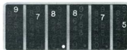
Fig. 8. New arrangement of column-type readout is shorter vertically and easier to read.
