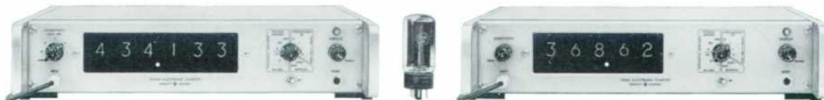
Fig. 1. New -hp- 1.2-megacycle and 300-kilocycle general-purpose frequency counters are designed to display measurements in a non-intermittent type readout that eliminates usual visual interruptions in readings. Counters are also arranged to measure low frequencies by averaging up to 10^5 periods,
