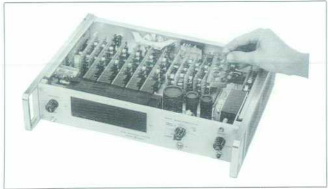
Fig. 10. Circuitry in new counters is built in plug-in modules.
