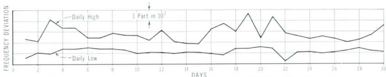
Fig. 3(a). Long-term accuracy curve measured of time base in 1.2-megacycle counter. Excellent long-term stability for a counter of this class has been achieved by operating time-base crystal near room temperature. Short-term variations in curve are largely due to ambient temperature variations.
