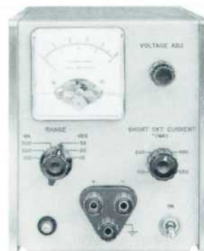
Fig. 2. New -hp- Model 723A regulated power supply provides up to \frac{1}{2} ampere at voltages from 0 to 40 vdc. Unit is fully transistorized and operates at full ratings up to 55°C as does new supply at left. Unit is programmable and has current-limiting feature.
