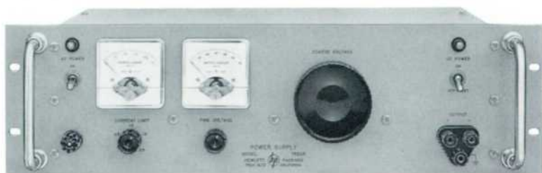
Fig. 1. New -hp- Model 722AR regulated power supply provides up to 2 amperes at voltages from 0 to 60 vdc. For safety to load, maximum available current can be set anywhere between 100 ma and 2.2 amperes. Unit is also designed to compensate for effect of hook-up leads on regulation. A companion version of unit is designed to be remotely programmable.
