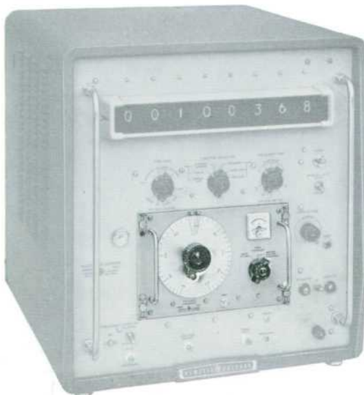
Fig. 1 (at left). New -hp- Model 525C Frequency Converter panel plug-in unit operates with -hp- 524B/C/D counter to measure frequencies from 100 to 510 megacycles with accuracy of counter itself. Converter unit is fully transistorized.
