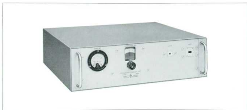
Fig. 1. New Microwave Frequency Doubler enables existing lower-frequency signal sources to provide signals in the 18-26.5 kmc or 26.5-40 kmc ranges.
