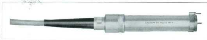
Fig. 15. Physical form of signal probe. Each channel of plug-in unit is equipped with one such probe on five-foot cable.
