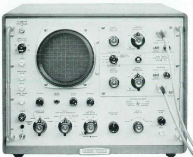
Fig. 6. Panel view of hp Model 185A Oscilloscope with Model 187A Dual-Trace plug-in amplifier. Instrument uses new circuit technique, but controls are conventional and include presentation selector for separate or combined - channel displays.
