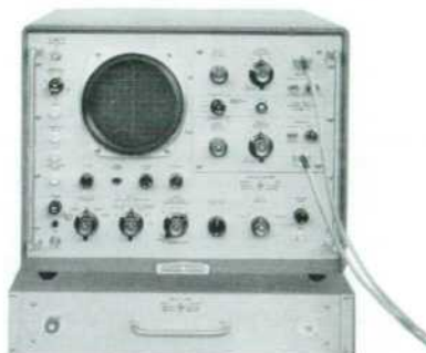
Fig. 13. hp AC-16V Delay Line can be used to delay triggering of external circuit or to delay signal, is arranged to fit out of the way under oscilloscope.
