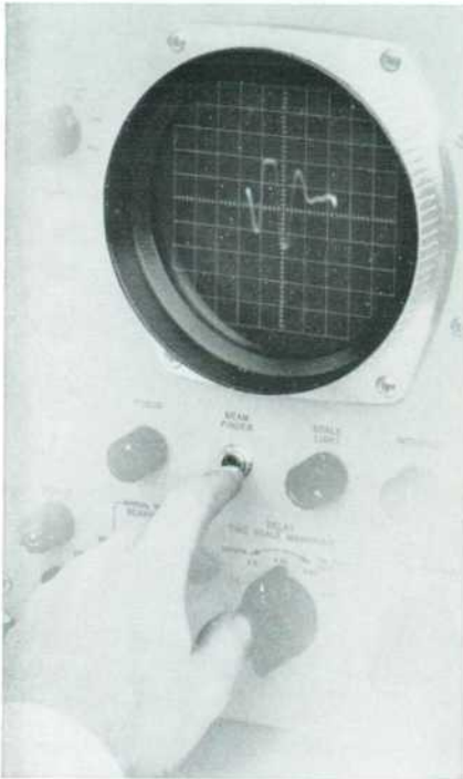
Fig. 3. New "beam-finder" feature enables off-screen trace to be located immediately by pushing panel switch, thus overcoming long-time oscilloscope inconvenience. When switch is depressed, display indicates direction and amount beam is off-center, greatly simplifying adjustment of centering controls.
