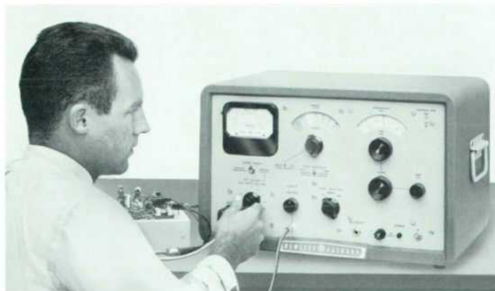
incorporates AFC circuit and linear tuning dial to simplify tuning. Voltage-measuring range extends below 10 microvolts. Instrument has sine wave output at dial frequency to facilitate transmission tests on external circuits.
