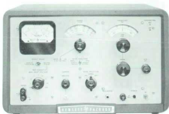
Fig. 4. Panel view of analyzer. Constant-resolution tuning dial appears in right-hand panel window. Fine tuning control drives tuning capacitor through 100:1 reduction gear train giving dial length of more than 50 feet.
