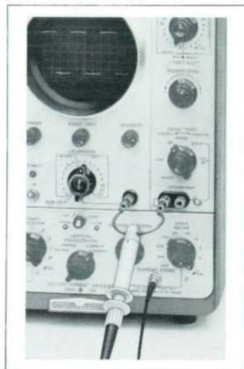
Fig. 11. Amplitude and phase response of probe and amplifier can easily be checked using calibrator on Model 150A Oscilloscope.
