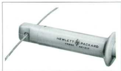
Fig. 4. Current probe clips around conductor to make measurement. Probe jaws are operated by flanges on probe body and accept conductors up to 0.175-inch O.D.
