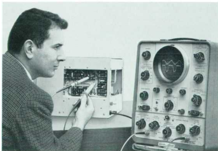
ternating currents as small as 1 ma and up to 8 mc in frequency to be measured merely by clipping probe on conductor. Unit also includes voltage channel and dual-trace provision to permit voltage to be measured simultaneously with current.
