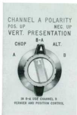
Fig. 3. Vertical presentation selector provides for five types of vertical display. Concentric switch inverts A channel signal to facilitate two-signal comparison.
