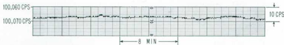
Fig. 2 (above). Typical stability characteristic of -hp- Model 200T operating at its highest rated frequency of 100 kc after warmup. Even higher percentage stability will usually be obtained at other output frequencies (see Fig. 3).
