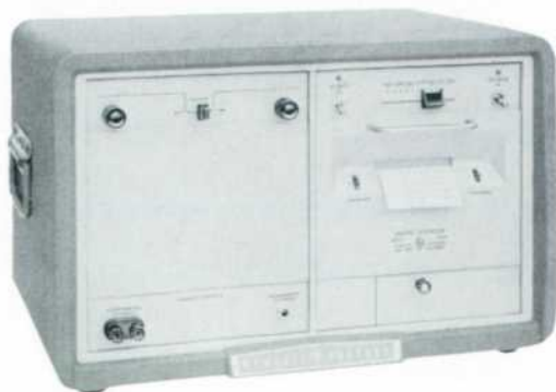
Fig. 1. New hp Model 560A Digital Recorder prints hp electronic counter readings on paper tape at rates up to 5 lines per second and up to 11 columns per line. An important feature of the instrument is that it provides output voltages proportional to the counter reading so that counter readings can be simultaneously and automatically plotted by strip recorders.
