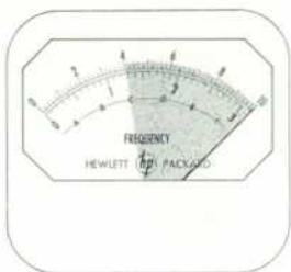
Fig. 3. Same shift as in Fig. 2 will cause pointer change shown when measured in \times 10 expanded operation.
