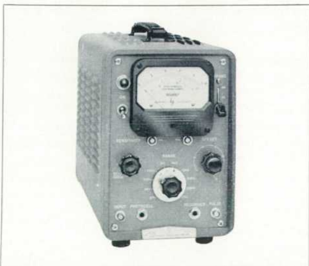
Fig. 1. New -hp- Model 500B Electronic Frequency Meter measures frequencies from 10 cps full scale to 100 kc full scale in 9 ranges. Special features include a discriminator output for measuring f-m and the ability to expand its scale for increased accuracy in frequency change measurements.
