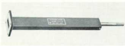
Fig. 1. -hp- Model X914A Sliding Load permits measurement of "residual" VSWR of transmission system to obtain more accurate VSWR measurements.
