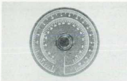
Fig. 3. Dial used on -hp- Model 200I Spread-scale oscillator.
