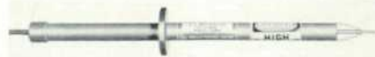
Figure 11. -hp- Model 459A Multiplier permits measurement of voltages up to 30,000 volts d-c.
