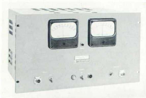
Figure 1. -hp- Model 520A High-Speed Scaler operates up to 10 mc.
