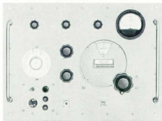
Figure 1. Panel view of -hp- Model 618A 3800-7600 Mc Signal Generator.
