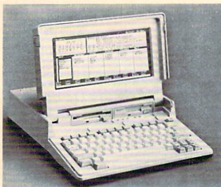
Laptop power: Tandy's new 1400 LT offers PC compatibility, 768K of RAM, two microfloppy disk drives, a backlit supertwist LCD screen, and removable battery pack—all for $1,599.
