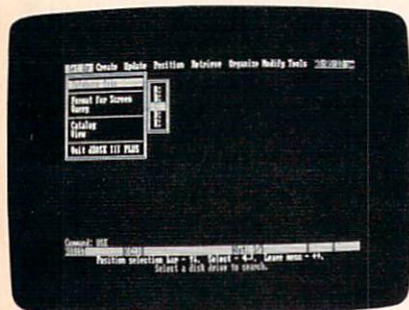
IBM's original monochrome display adapter (MDA) provides very readable text, but no true graphics or color capabilities.
