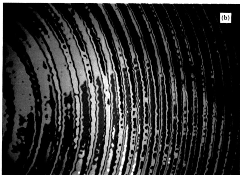
Fig. 11—Slab sample from tip of optical fiber preform showing improved rendering of layer structure achieved with video colorization.
