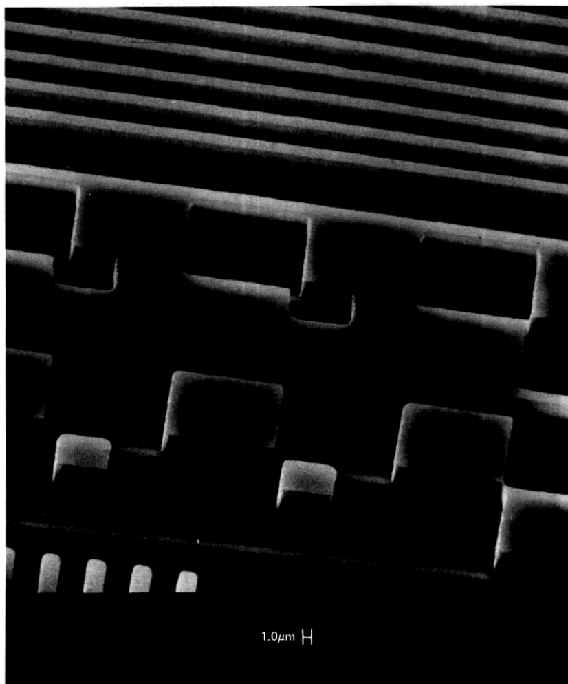
Fig. 4—Pattern sputter-etched using a system having no exposed metallic surfaces. Etching has caused no fiber formation.
