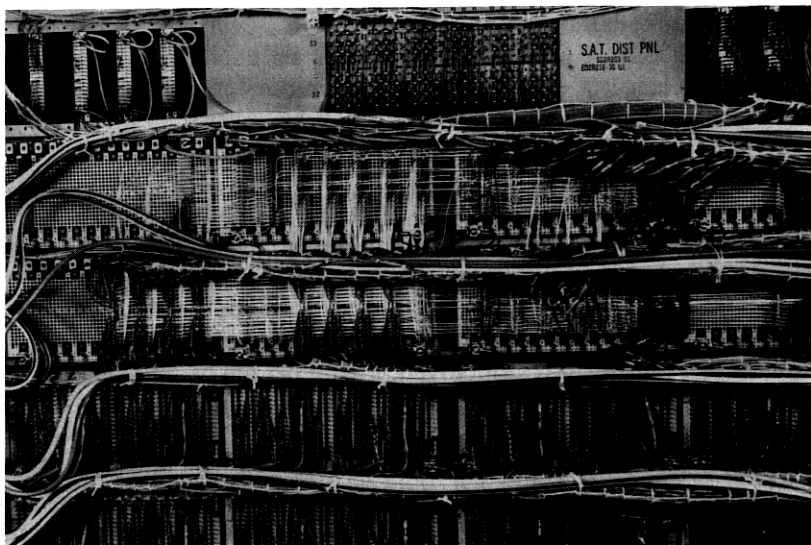
Fig. 21—Backplane wiring showing both local wiring and interpanel cabling.
